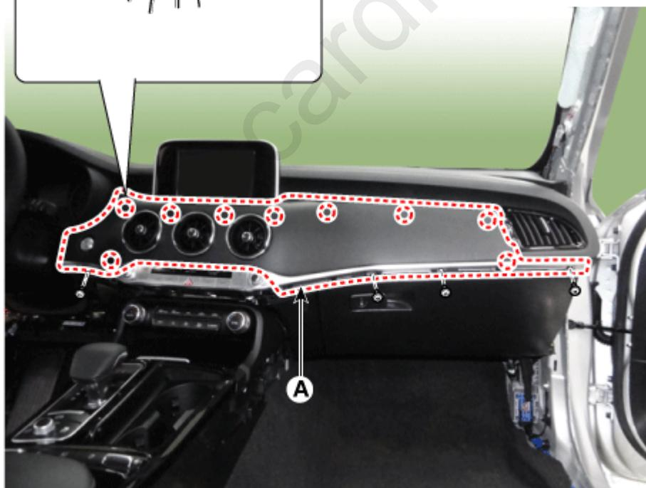
4. Disconnect the start/stop button connector (A) and then remove the crash pad garnish.
