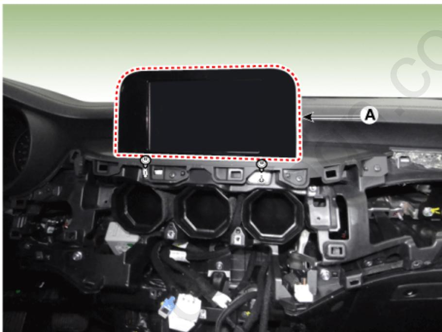
6. Remove the monitor assembly (A) after disconnecting the connectors.
