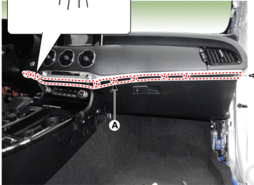
3. Separate the crash pad passenger side panel (A) after loosening the mounting screws.
