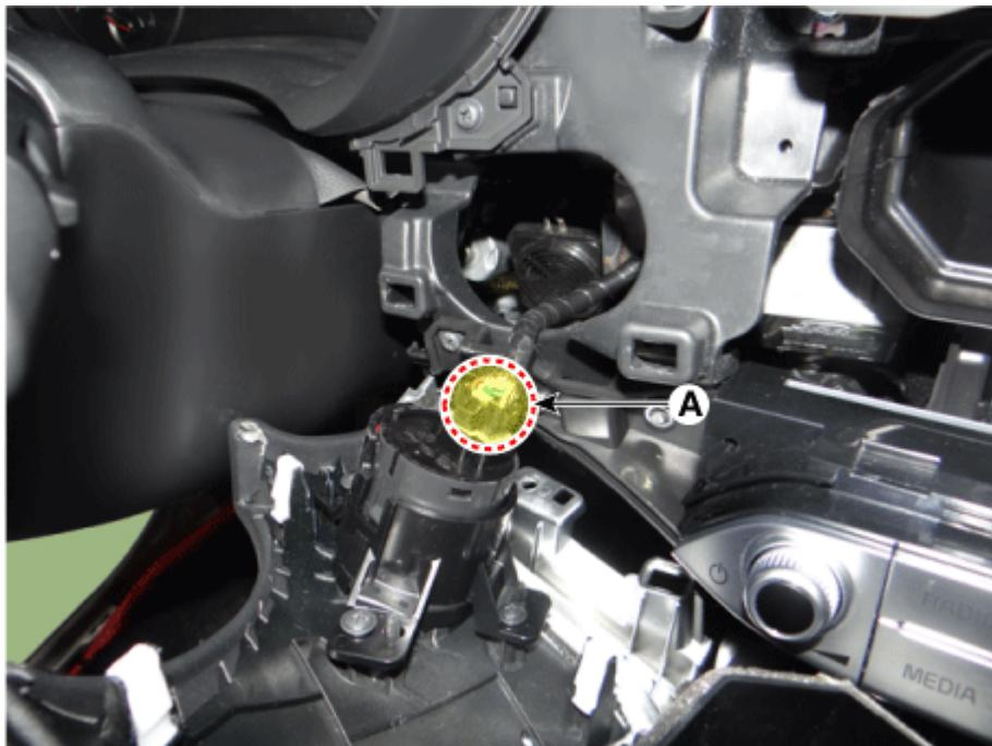
5. Separate the monitor assembly (A) after loosening the mounting screws.
